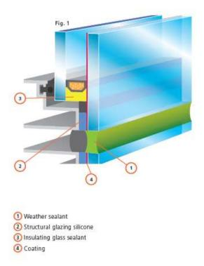
For the so called 'stepped insulating glazed units' or insulating glazing with 'integrated mechanical fixings in the sealant joint', two points have to be respected:
