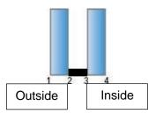
Planibel Easy Clear and Easy Blue can be assembled in insulating glazing units (IGUs) with the following restrictions on the position of the coated surface.
