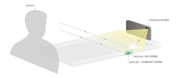
**Coated side up**: The green spot is on top and the white spot underneath.
