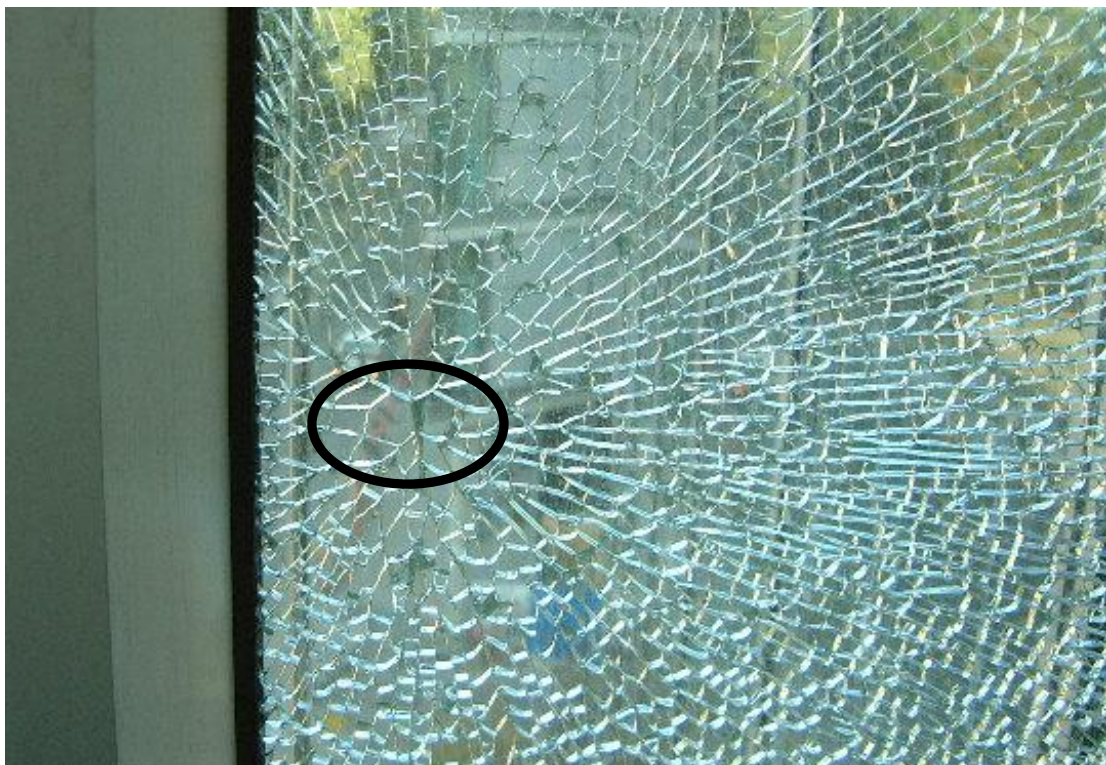
Typical breakage starting from a NiS inclusion
