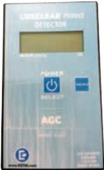
Another method for determining the coated side is using an AGC Coating Detector which is also available on [www.agc-store.com](http://www.agc-store.com).
