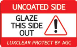
As Luxclear Protect is a non-conductive coating and cannot be detected by conventional means, the glass should be marked with stickers (labels) on the non-coated side. Processors can buy Luxclear Protect stickers on [www.agc-store.com](http://www.agc-store.com).
