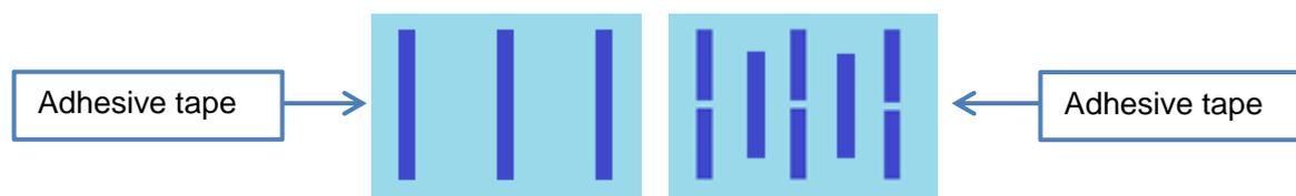
AGC Glass Europe recommends using ten 10 mm x 100 mm strips per kg of mirror and to apply several smaller pieces rather than one single length (as indicated above).
