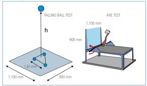
In falling ball tests, a test sheet measuring 1,100 mm x 900 mm is positioned horizontally and is impacted by a ball weighing 4.1 kg in a triangular area in the centre of the glass (13 cm between impacts). The impact number and the drop height vary depending on the class.
