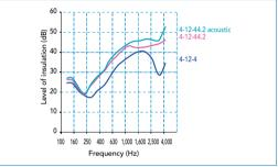
The direction in which dissymmetrical double glazing and/or double glazing with laminated glass are installed has no effect on the acoustic performance of the glazing. It is advisable to position any laminated glazing with the PVB on the inside to ensure safety in the event of breakage.
