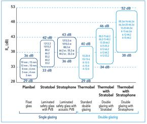
At equivalent levels of acoustic performance, Stratophone compositions are thinner than Stratobel ones. In practice, this means, for example, that to achieve a performance level ( $R_w$ ) of 36 dB, either a Stratobel 66.2 or a Stratophone 33.2 glass may be used.
