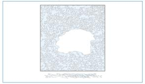
Thermally toughened glass is considered to be a safety glass if it meets the relevant break pattern criteria. These criteria are set out in standard EN 12150, which also describes the test to be carried out to ascertain this break pattern.
