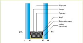
Insulating glazing: components and numbering of the sides
