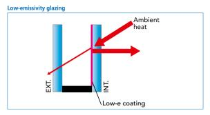
The conventional metal spacer made out of aluminium or steel can on demand be replaced by a warm-edge-type spacer (which can be reinforced by a metallic structure in some cases). The thermal conductivity of warm-edge-type spacers is far superior to that of steel or aluminium and thus reduces heat loss through the edges of the glass.
