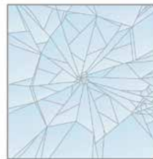
Example of fragmentation of laminated glass
