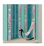
Start installation at outer edge. Position and adjust the sheet whilst floating on silicone.
