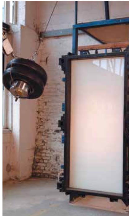
SOFT BODY IMPACT TEST
