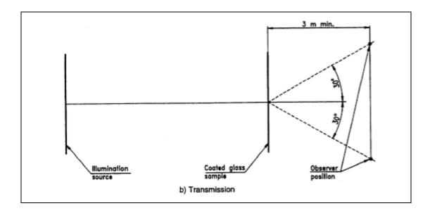
For panes of coated glass in finished sizes ready to be installed, both main area and edge area of the pane shall be examined (see figure).
