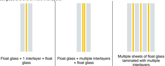
The Stratobel and Stratophone ranges can be used for safety and sound insulation purposes and can be installed indoors and outdoors.
