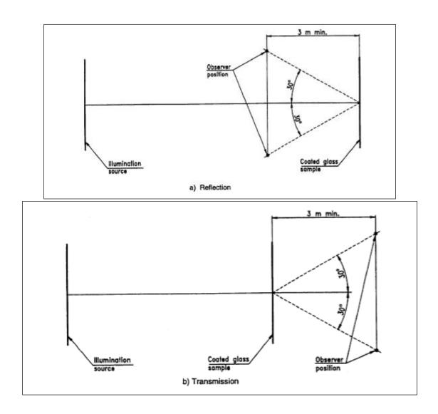
For panes of coated glass in finished sizes ready to be installed, both main area and edge area of the pane shall be examined (see figure).
