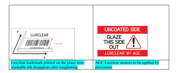
As glass coated with Luxclear cannot be visually distinguished from normal float glass, panes coated with Luxclear must not be stored or transported mixed with normal float glass - in order to avoid subsequent identification issues. In any case, it is important that the uncoated surface is labelled with the correct Luxclear sticker after cutting.
