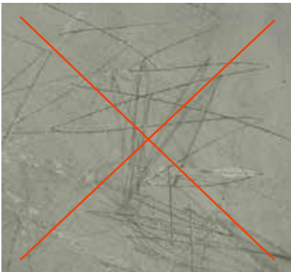
WRONG: CLEANING WITH DIRTY AND DRY CLOTH
