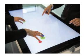
AGC's TIREXtreme glass is a clear float glass with very high transmission in the near-infrared range, optimised for wave-guiding applications. This makes it the material of choice for any application dealing with near infrared and the perfect solution to implement infrared in-glass touch technologies in large displays.
